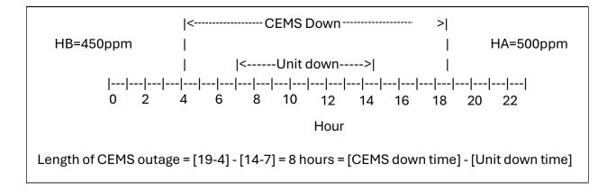
Assume that the PMA of the  $SO_2$  monitor is  $\geq 95\%$ . As illustrated above, the missing data period is 8 hours, when the unit downtime is excluded. Therefore, according to \$75.33(b)(1)(i), the appropriate substitute data value to fill in gaps from hours 4 to 7 and hours 14 to 19 is the average of the hour before and hour after values, i.e., (HB + HA)/2 = (450 + 500)/2 = 475 ppm.
