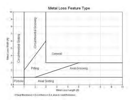
Metal Loss Feature Type graphic adapted from the Pipeline Operators Forum [POF] Metal Loss Definitions
