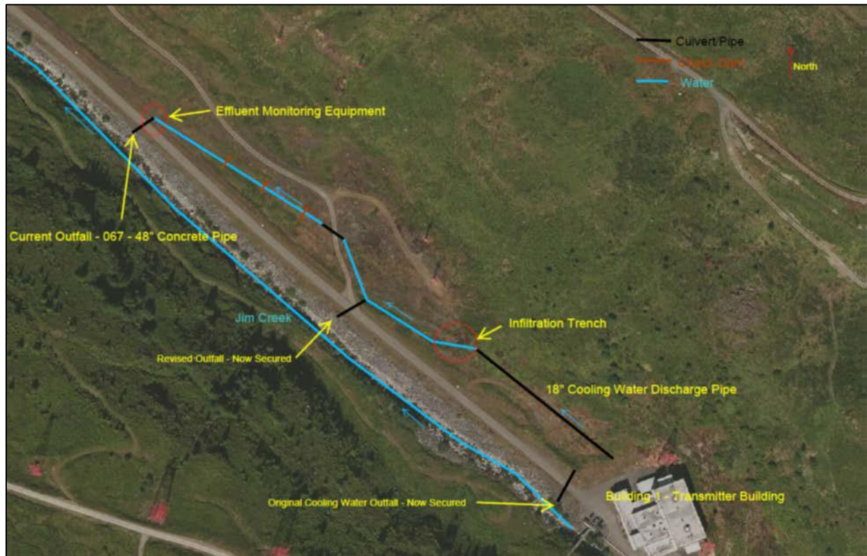
Figure 1. The Jim Creek Naval Radio Station transmitter building and outfall location in relation to Jim Creek.
