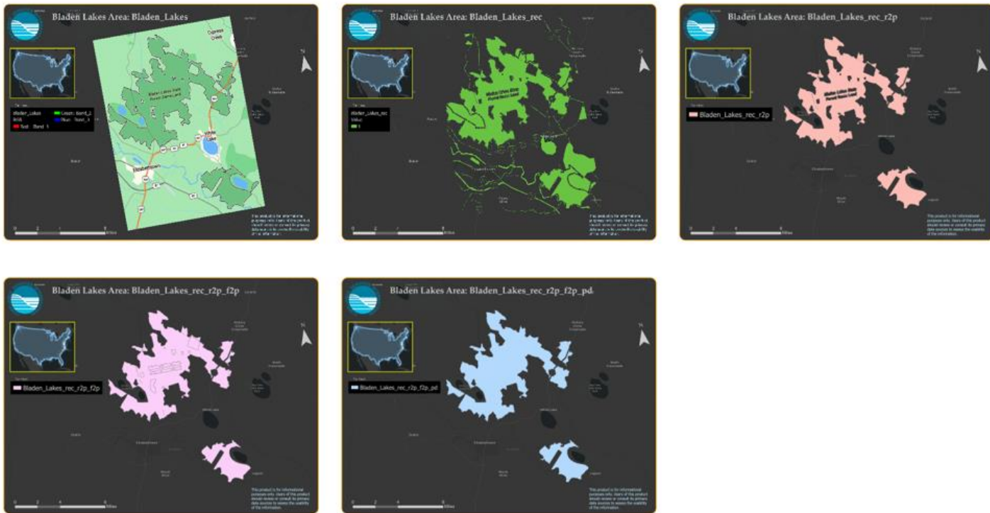
Figure 5. Core map extent for Bladen Lakes area. An image of the Bladen Lakes area (top-left) was reclassified (top-center), converted to a polygon layer (top-right), had its holes filled in (bottom-left), and dissolved into a single shape (bottom-right).
