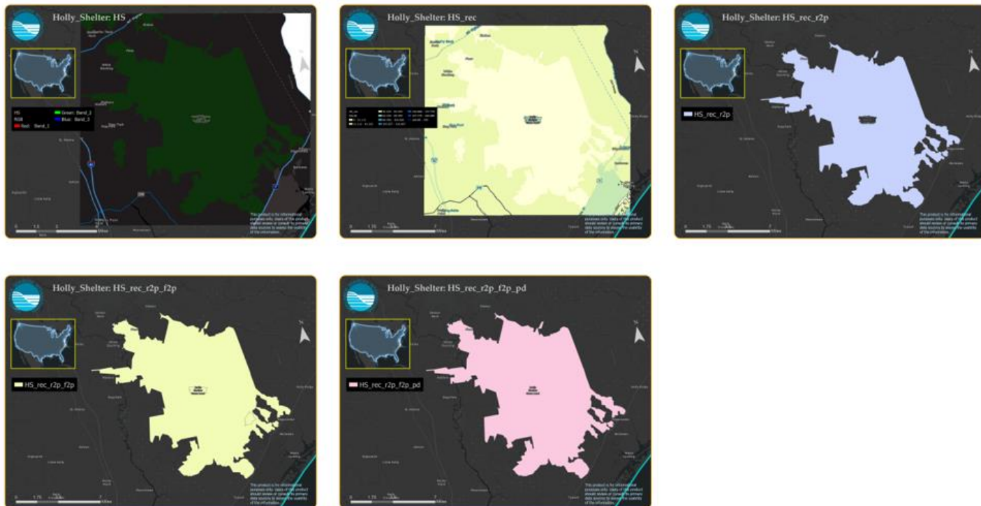
Figure 11. Core map extent for the Holly Shelter Game Lands. An image of the Holly Shelter area (top-left) was reclassified (top-center), converted to a polygon layer (top-right), had its holes filled in (bottom-left), and dissolved into a single shape (bottom-right)
