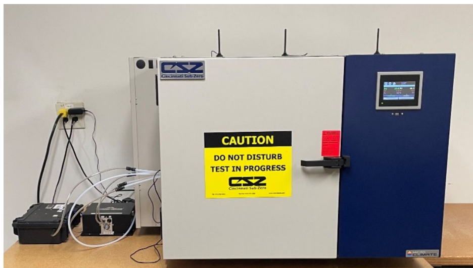
Figure A-1. The chamber and sampling setup or the lab-based verification.
