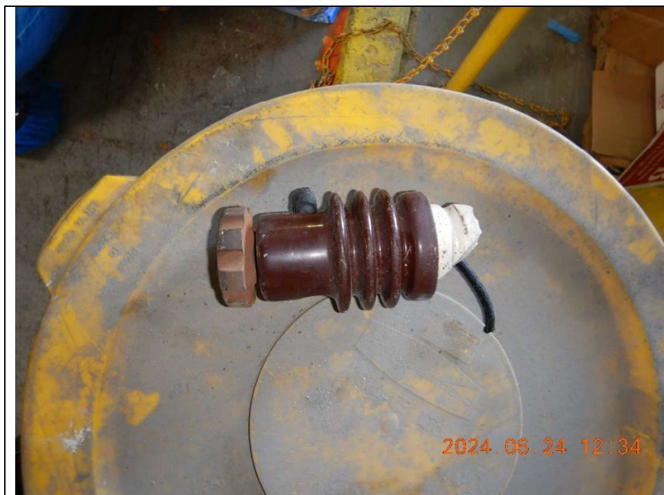
Photograph 43. Sample location for wipe sample 24264403, which was taken from the inside of the broken bushing found in the waste receiving area.
