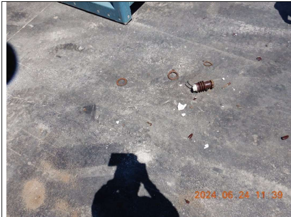
Photograph 32. Broken bushing observed in waste receiving area.
