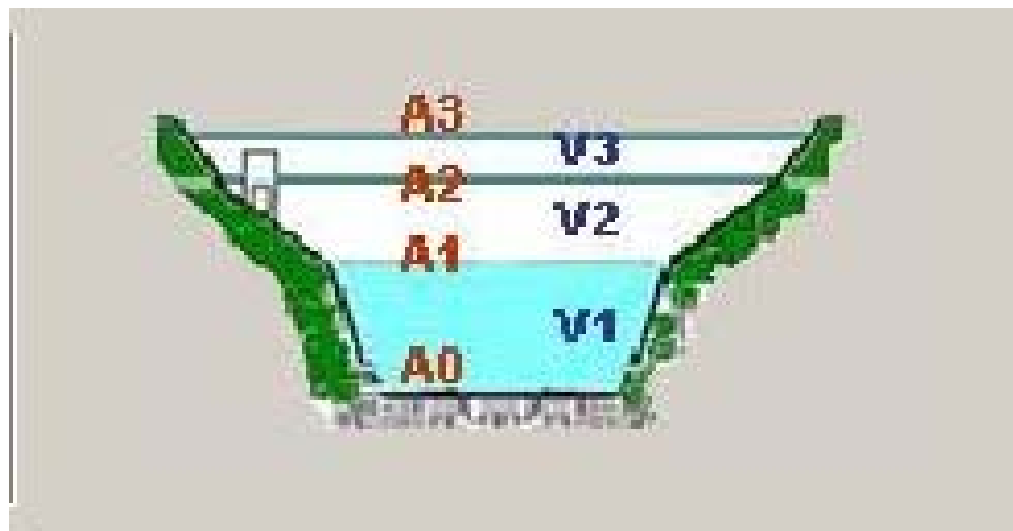
Figure 4-34. The BMPDSS multi-stage pond module.
