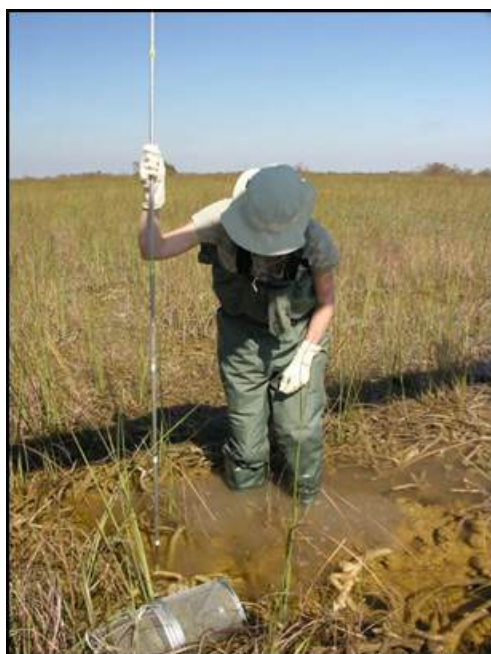
Photo 14. Soil thickness measurements were collected with a soil rod.
