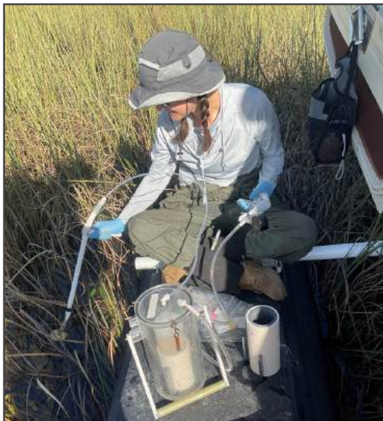
Photo 8. Water samples were filtered and collected using a specially designed vacuum chamber.
