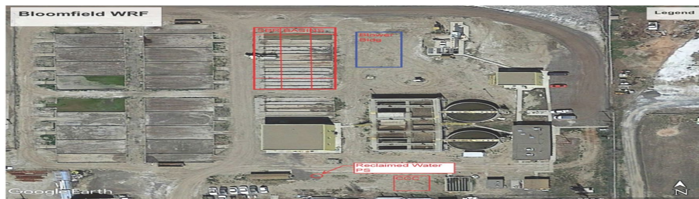
Aerial image 3: Overall view of the existing City of Bloomfield's Wastewater Treatment Plant and the upgrades denoted in "red". Aerial from Google Earth.
