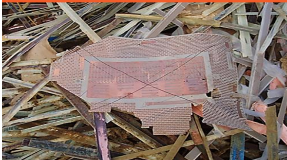
Circuit board waste with high levels of copper and other metals impacted soil and water at the site. (photo credit: EPA)
