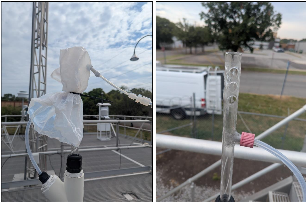
Figure 9-8. Soft Connection (left) to Station's Glass Tubing Sampling Inlet (right)
