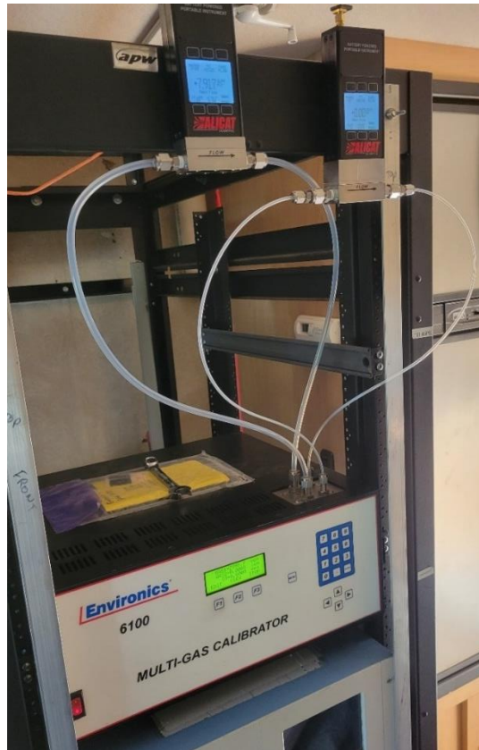
Figure 7-4. Alicat Flow Rate Transfer Standards Plumbed in-line with an Environics® 6100 Gas Calibrator
