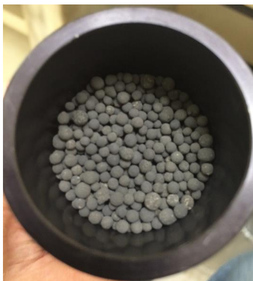
Figure A-3. Addition of Palladium Coated Pellets
