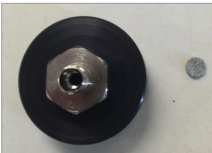
Figure A-1. Removing Frits from End Caps
