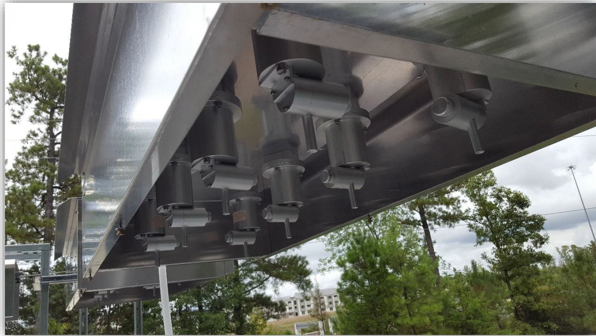
Figure 1. One of four sampling manifolds on the 32-cyclone collocated PE sampler at OSAP in RTP, NC.
