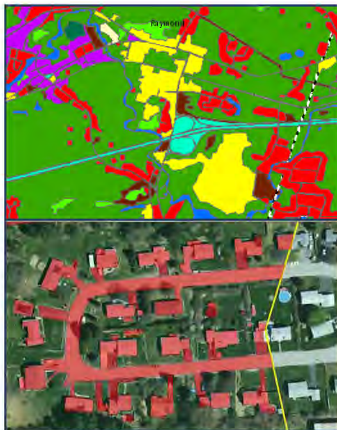
Figure 1. EPA will use statewide land use data (GRANIT), subbasin boundaries, and land use impervious coefficients to estimate baseline IA for each MS4 jurisdiction (upper). Communities may choose to refine these estimates with direct measure of IA where local GIS capacity is available, as shown here from Somersworth, NH (lower).
