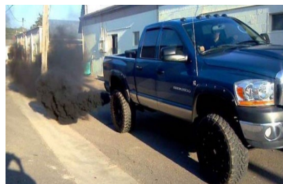
A vehicle with defeated emissions controls releases hazardous smoke, also known as “rolling coal,” into the air. (EPA image)
