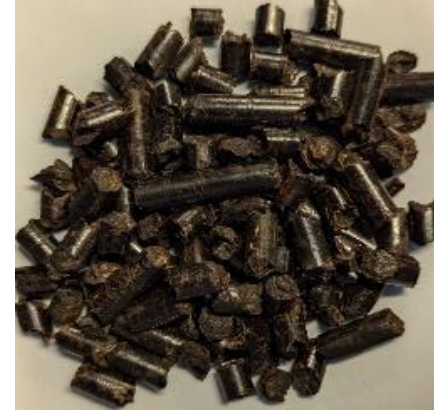
Corn stover pellets that resemble the heating value and particle size qualities of coal
