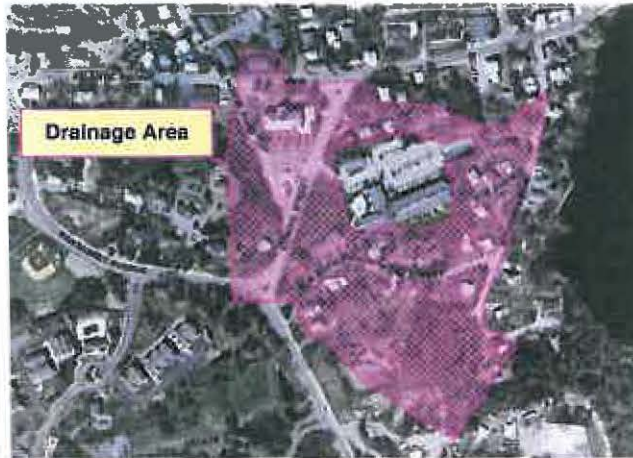
DRAINAGE AREA FOR STORMWATER TREATMENT
