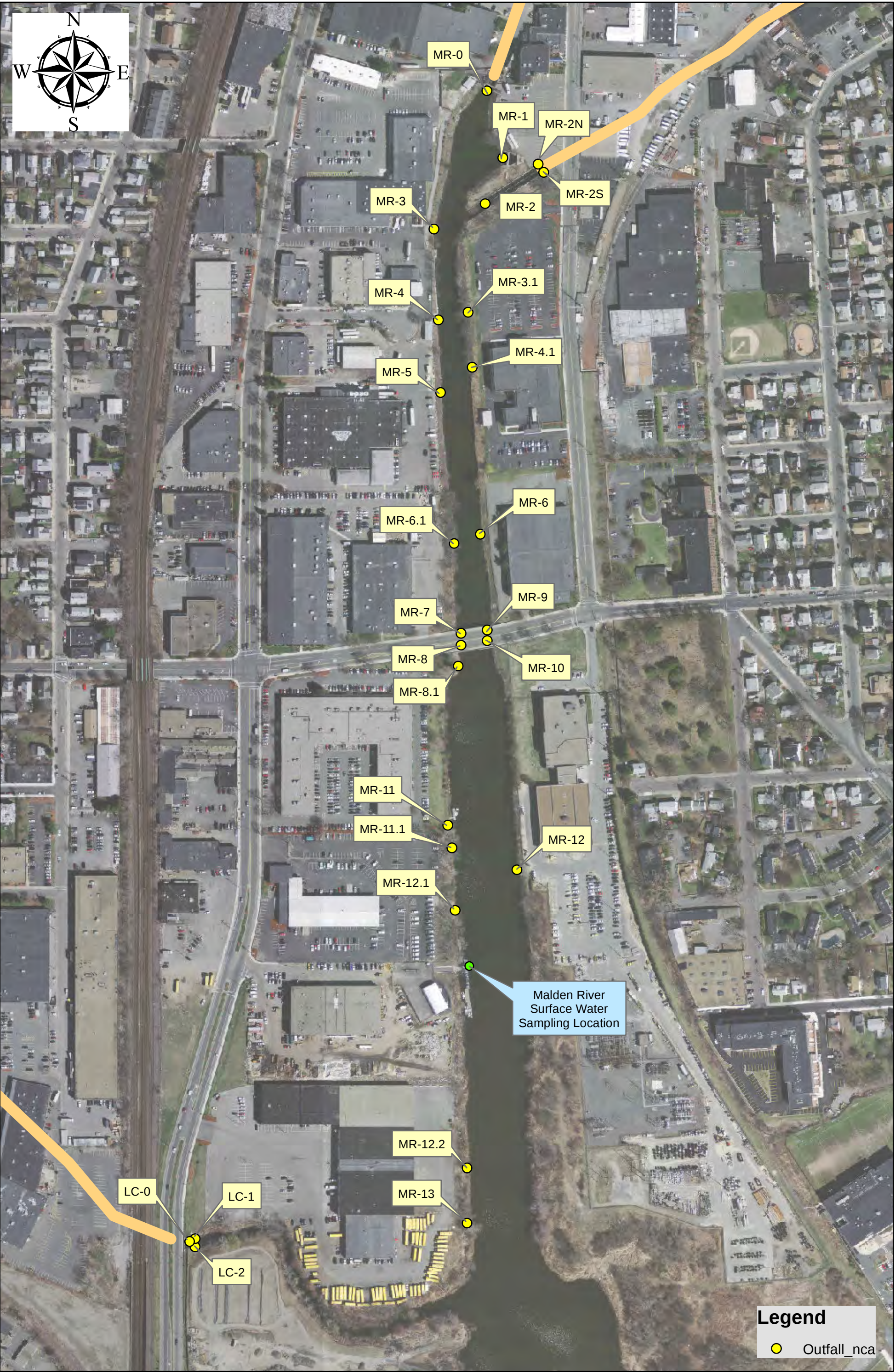
Figure 5 - Malden River Outfalls
