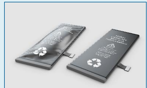
Figure 2. Swelling is a sign of damage and defects in lithium batteries and can precede battery fires. Source: iStock
