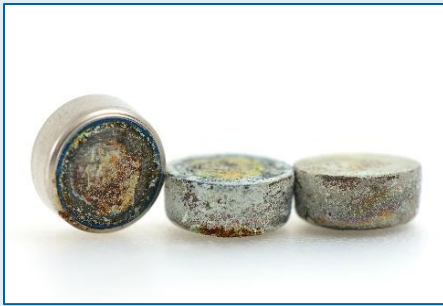
Figure 1. Left: Corrosion indicates damage in small format batteries such as button cell batteries. Middle: Smoke, leaking and odors may indicate damage and defects. Right: Discoloration of small format batteries may indicate damage. Source: iStock
