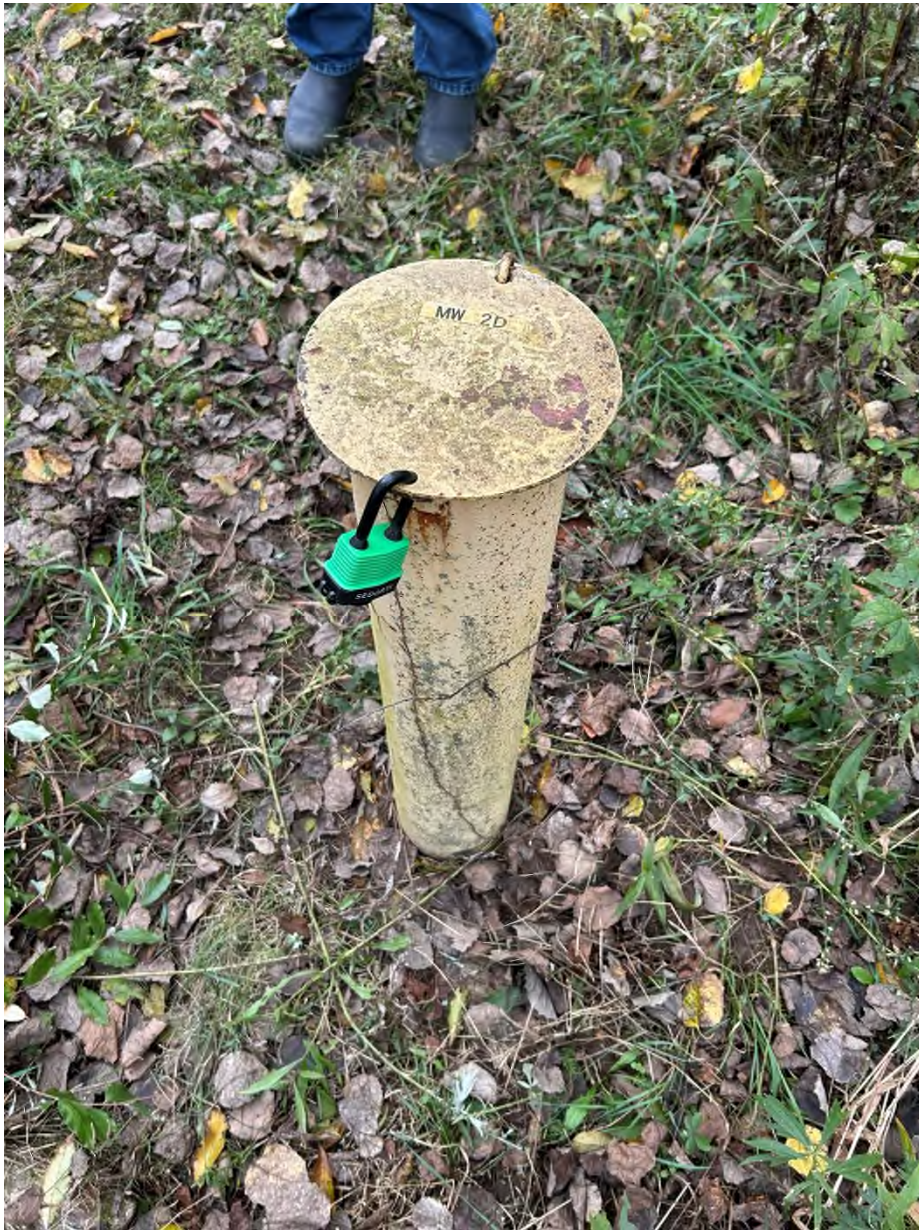
Figure 5: Image of the well MW-2D as seen during the site walk.
