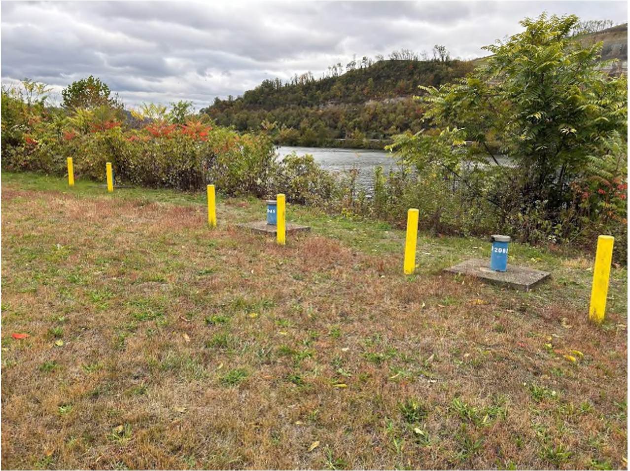
Figure 11: A cluster of monitoring wells (R-208D, R-208I and R-208S) with Ohio River just southwest of the tree-lined embankment.
