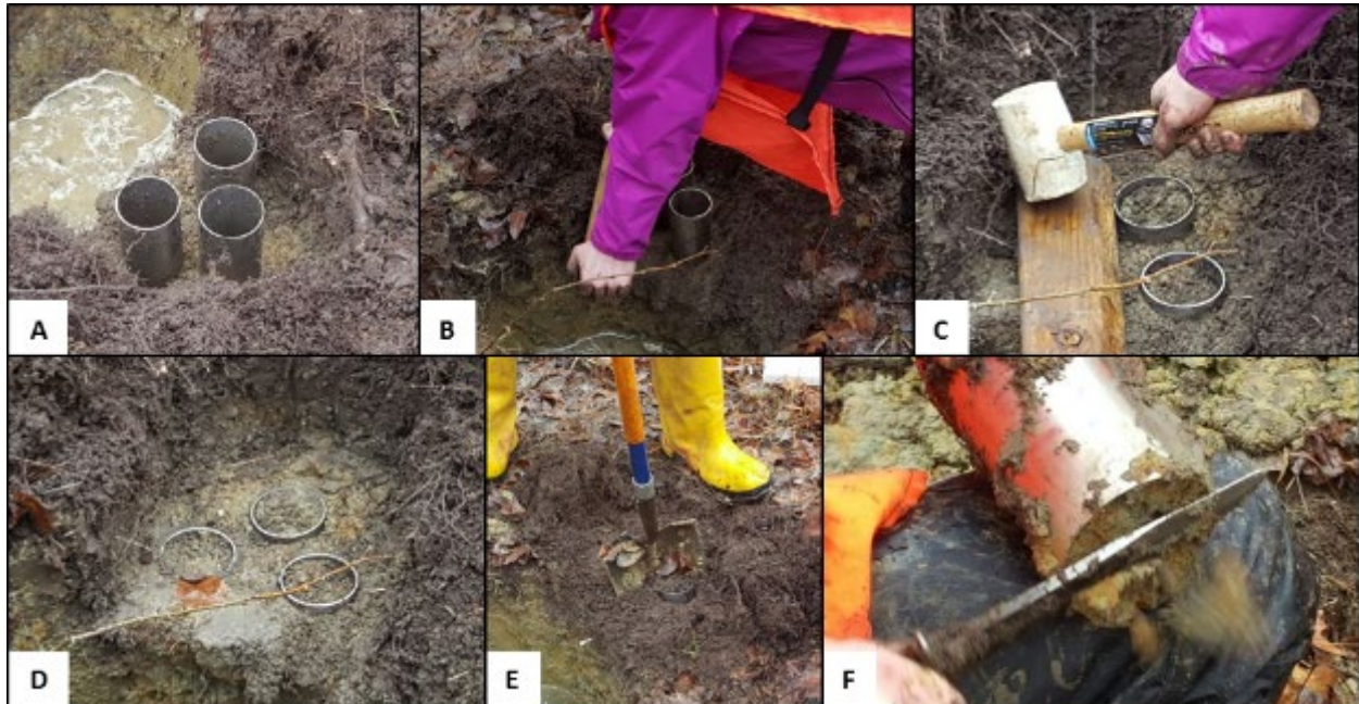
Figure 6-24. Demonstration of Soil Horizon Bulk Density sampling using the 3-in diameter stainless steel corers provided in the NWCA base kit. A) Smooth a planar horizontal area at the top of the horizon, then place the three open-ended corers (sharpened edge downward) on the surface (top of the horizon to be sampled); B-D) Push or gently hammer the core into the soil until the top of the corer is flush with the smooth surface; E) Dig out the corer plus some of the surrounding soil; F) Using a knife blade, cut off the excess soil so the sample material is flush with the bottom edge of the corer. Photos courtesy of Sarah Lehmann.
