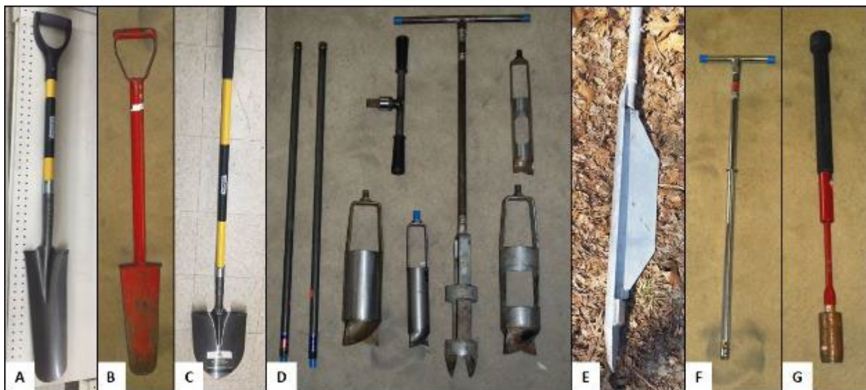
Figure 6-8. Examples of tools for Soil Pit excavation. A) Tiling spade. B) Sharpshooter. C) Shovel. D) (Left to right) Auger handle extensions, Ratchet handle, Solid auger buckets (for sand or mud), Open bucket auger with handle, and Open auger buckets (for fine textured soils). E) Peat auger head. F) Soil probe. G) Hammer corer. Photos by Frank Gibbs, Gregg Lomnick, and Phil King.
