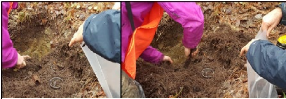
Figure 6-27. Collection of Soil Horizon Chemistry sample. Horizon Chemistry samples can be collected as Soil Horizon Bulk Density Sample cores are extracted. Photo courtesy of Sarah Lehmann.
