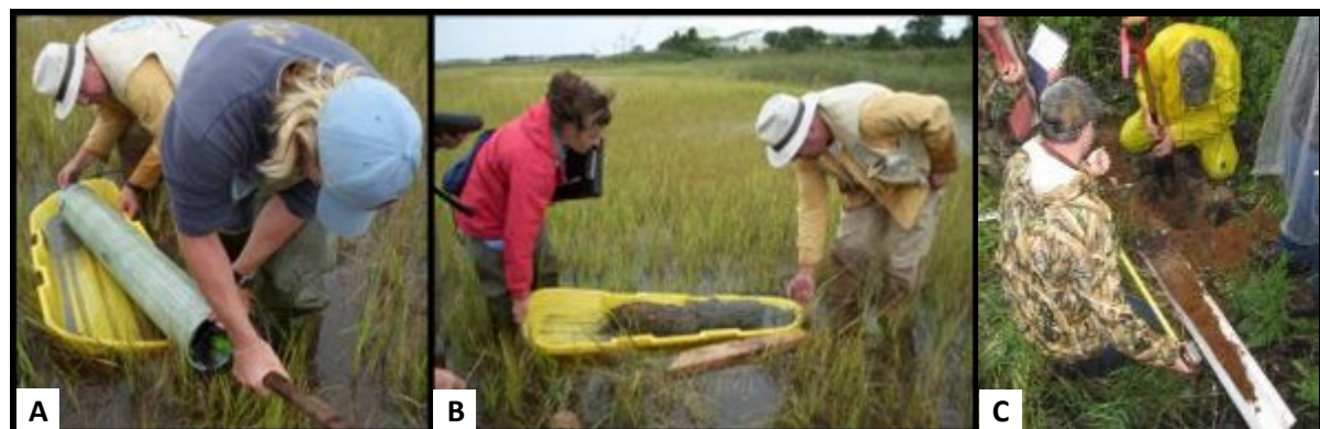
Figure 6-11. Use of a plastic snow sled (A and B) and plastic gutter (C) for facilitating sample collection and holding soil cores during soil profile description. Photos A and B by Regina Poeske. Photo C by Frank Gibbs.
