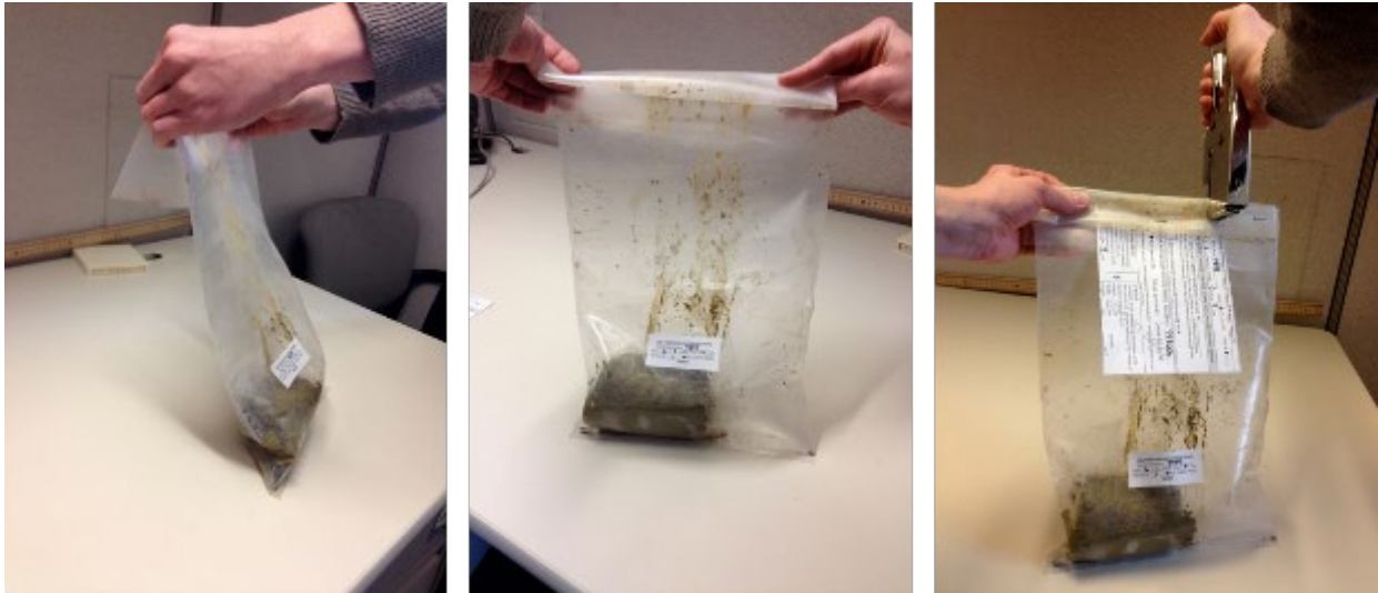
Figure 6-5. Proper sealing and stapling of soil sample bags
