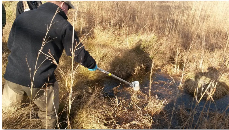
Figure 8-3. Example of long-handled dipper in use for sampling surface water. (Photo credit – Chris Turner, GLEC)
