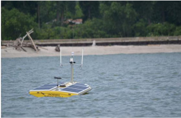
An uncrewed surface vehicle monitoring for algal toxins (left). An environmental sample processor (ESP) sits inside a custom underwater stationary mooring during deployment in Lake Erie (right). Source: NOAA.
