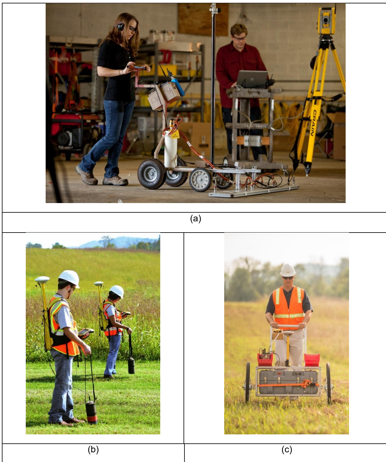
Figure 6-3 Various Human Manual and Pushed CCD Systems Used Indoors (a) and Outdoors (b)(c). (a) Gas proportional floor monitor survey using a total station for mapping indoor survey data, (b) a 2-in. by 2-in. Nal detectors integrated with Global Positioning System (GPS) equipment, (c) large-volume Nal detector integrated with GPS equipment. Image Credit: Oak Ridge Associated Universities
