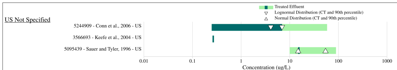
Figure 5-9. Concentrations of p -Dichlorobenzene (µg/L) in Wastewater in Treated Effluent from 1991–2004
