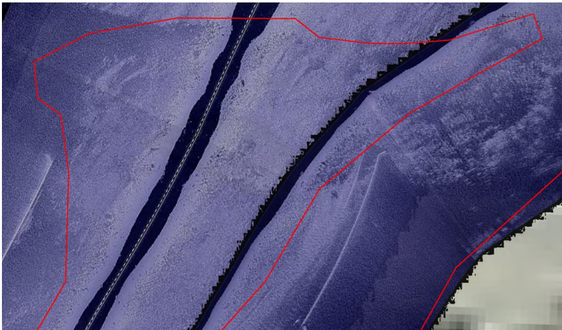
Figure 3-7. Example of gravel/cobble habitat type as classified from sonar imagery for the habitat survey of the Merrimack River, 16 September through 2 November 2010. (Note: gravel/cobble habitat is located within the bounds of the red polygon in the center of the figure).
