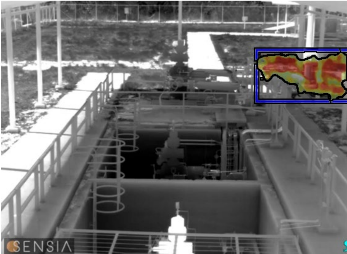
Figure 2: Example of an emissions plume detected by the SENSIA RedLook System MATM.
