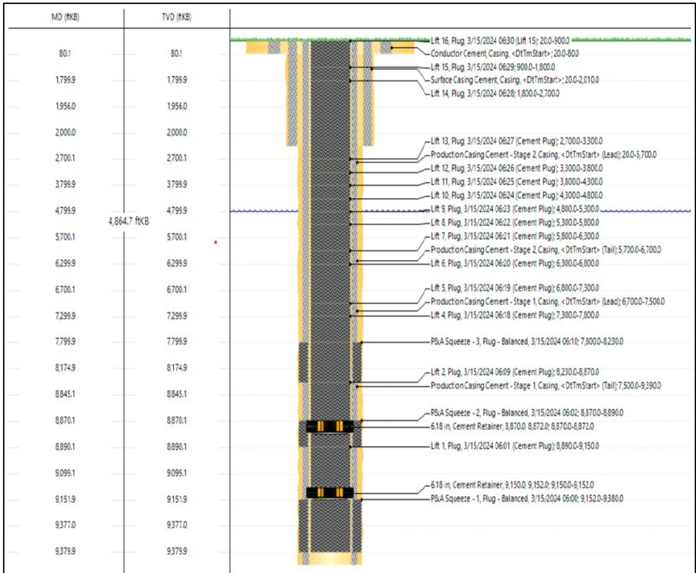
Figure 2: Front Range 2-1 well plugging schematic
