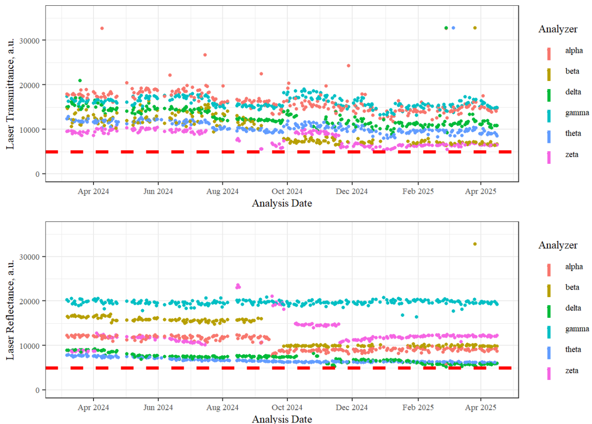
Figure 5-30: Laser initial readings (top: Transmittance; bottom: Reflectance) of the instrumental blank analysis for the analysis period 03/07/2024 through 04/17/2025 (samples collected 01/01/2024 through 12/29/2024).
