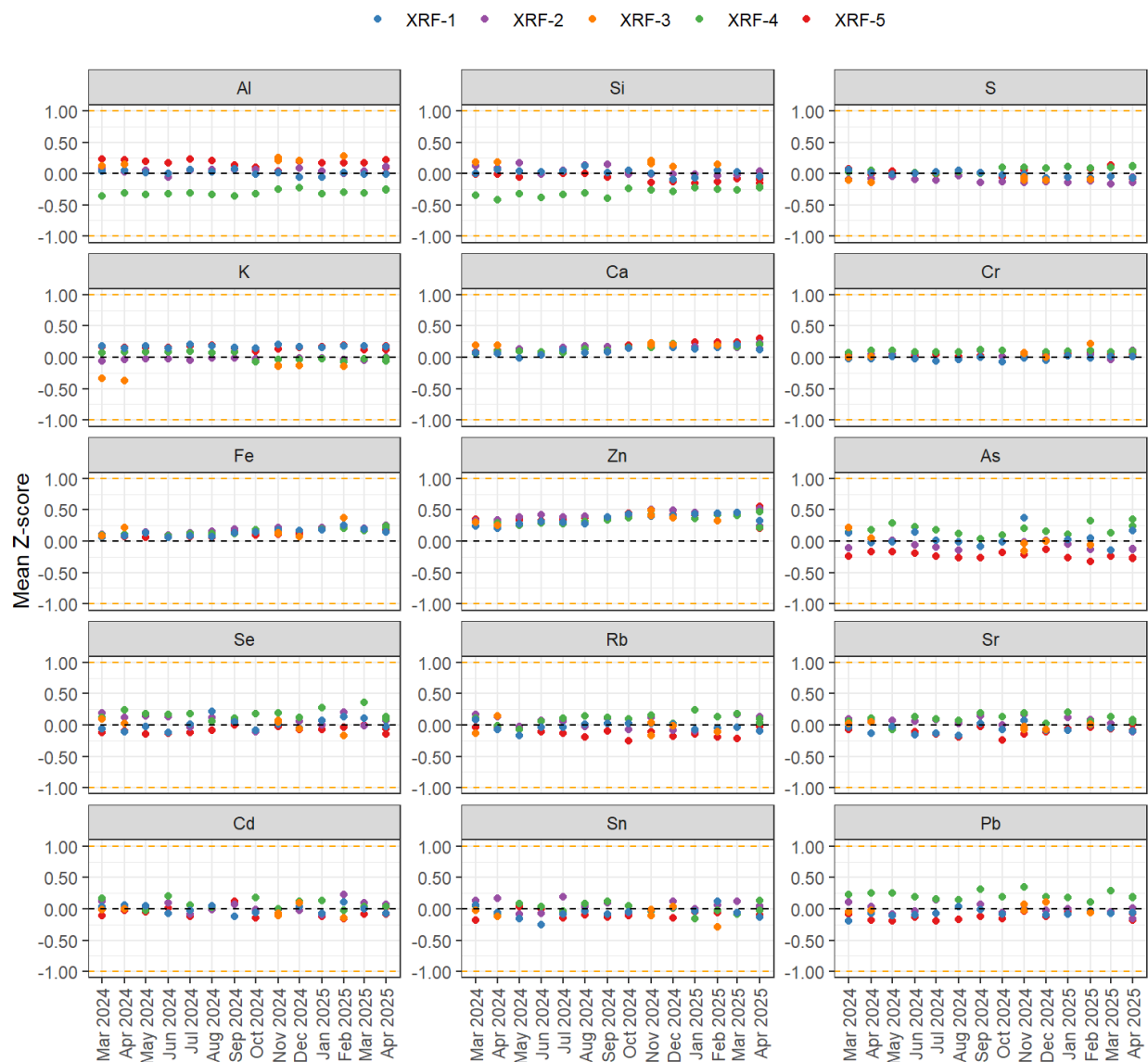
Figure 5-24: Inter-instrument comparison by z-score of monthly reanalysis sample set. The orange dashed lines indicate the mean z-score acceptance criteria of \pm 1 .
