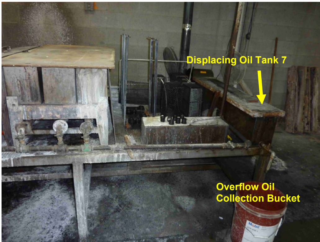
Figure 3 – Bluing Process - Displacing Oil Tank #7 and Oil Collection Bucket
