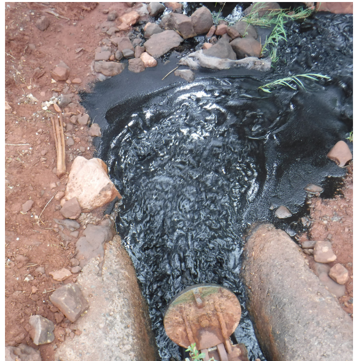
Fig 2: Manganese contaminants leaving a water system following ice pigging.
