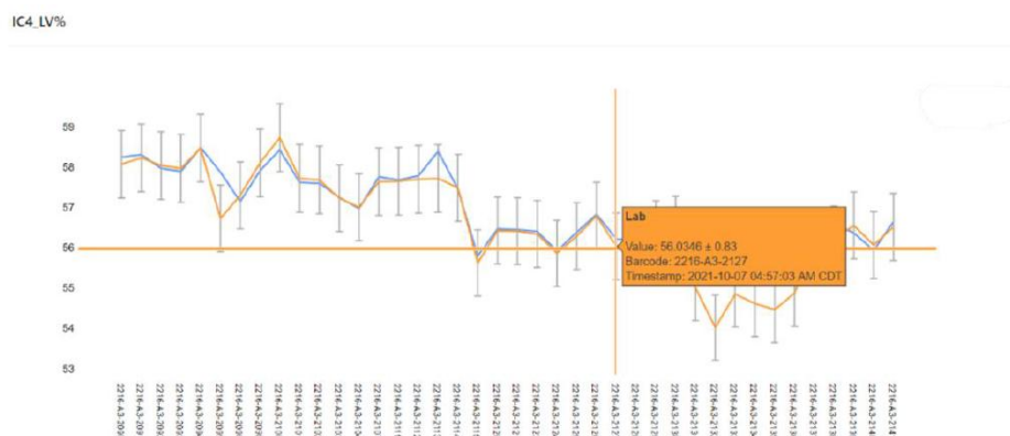
Figure 9: Example of iC4 validation samples collected over 18 months on a fractionation NGL stream tested via ASTM D6122
