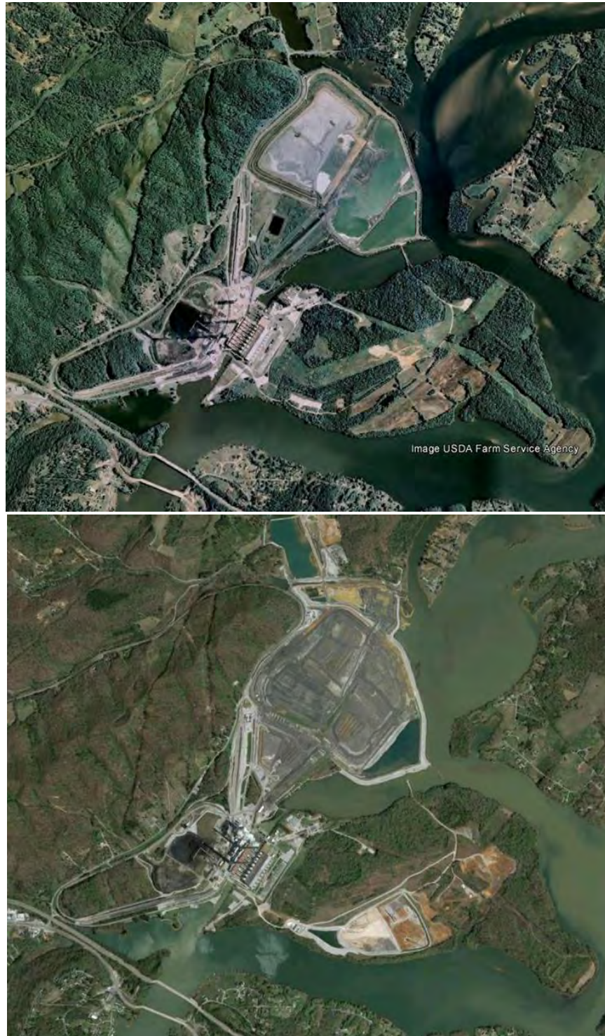
Figure 9-2: Kingston Fossil Plant in September 2007 (top), and in April 2013 (bottom). The ash spill occurred in December 2008. Note changes in the perimeter of ash disposal area, conversion of the ash pond to dry stacking, and construction of the gypsum disposal area on the southern peninsula.
