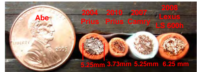
Comparison of Motor Leads
