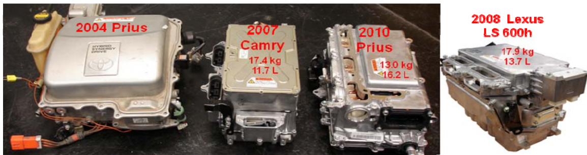
Fig. 2.2. Comparison of PCUs (which include motor and generator inverters).
