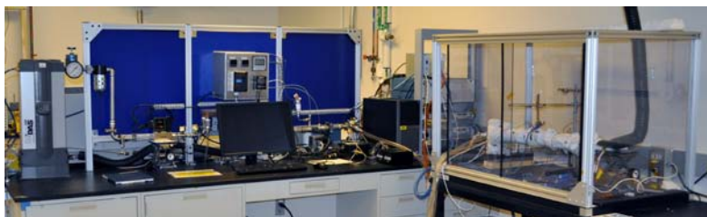
Figure V - 65: Photograph (left) and schematic (right) of the channel flow experimental setup: (1) compressed air, (2) desiccant dryer, (3) filter/regulator, (4) mass flow controller, (5) laminar flow element, (6) plate heat exchanger, (7) temperature control bath, (8) fin test section, (9) guarded heater, and (10) isolation box.
