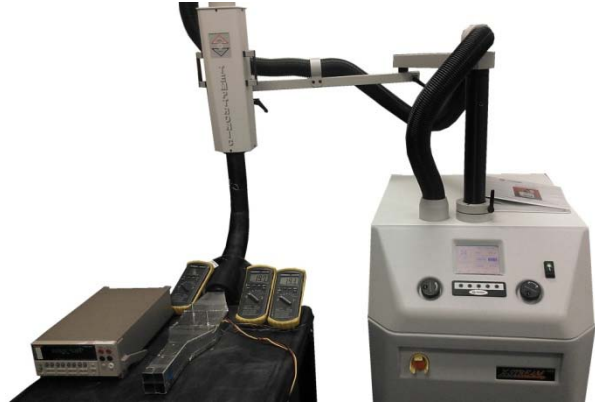
Figure II - 104: General test setup; Temprotronic X-stream 4310 air temperature and flow control (on right).
