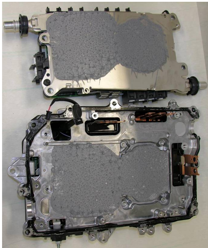
Fig. 2.9. Underside of power module/cooling structure (top) and bottom compartment (bottom).
