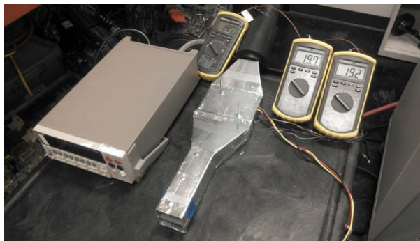
Figure II - 103: Temperature measurement devices and assembled test fixture.
