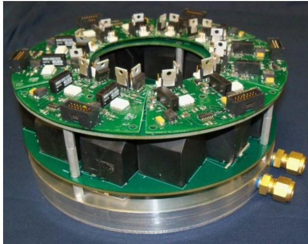
Figure II - 44: First 55 kW ring-shaped segmented inverter prototype using a four-channel toroidal heat exchanger.
