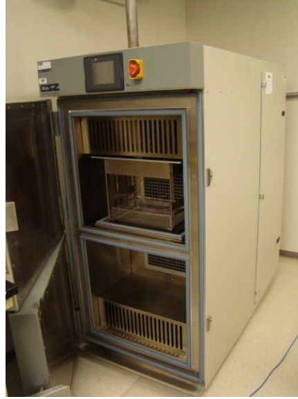
Figure 7. Thermal shock chamber
