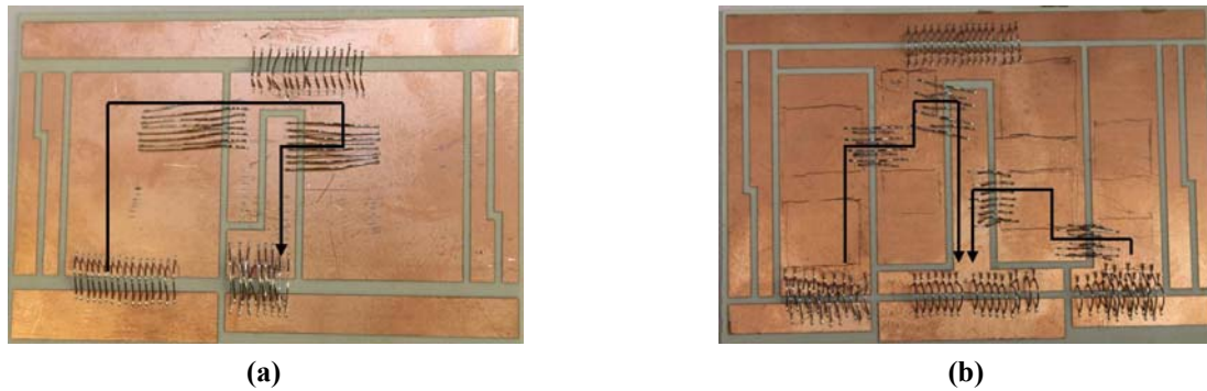
Fig. 15. Fabricated commutation loops for (a) the conventional design and (b) the proposed design.
