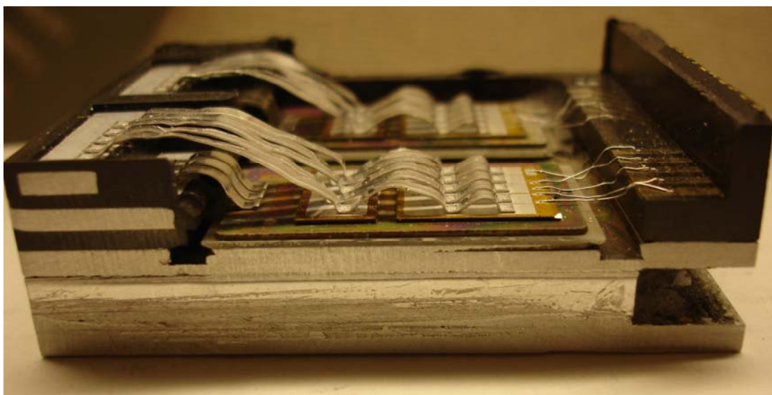
Fig. 2.20. Cross-section of boost converter modules 2010 Prius.
