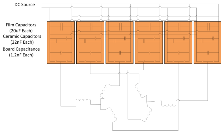
Fig. 7. Power circuit schematic for demonstrator 10 kW IMMD drive.
