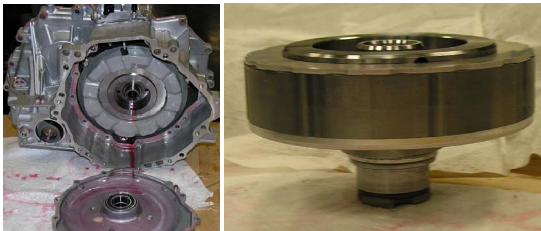
Fig. 2.64. 2010 Prius generator stator and rotor.
