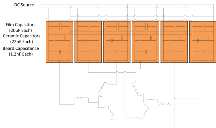
Fig. 8. Controller architecture for demonstrator 10 kW IMMD drive.
