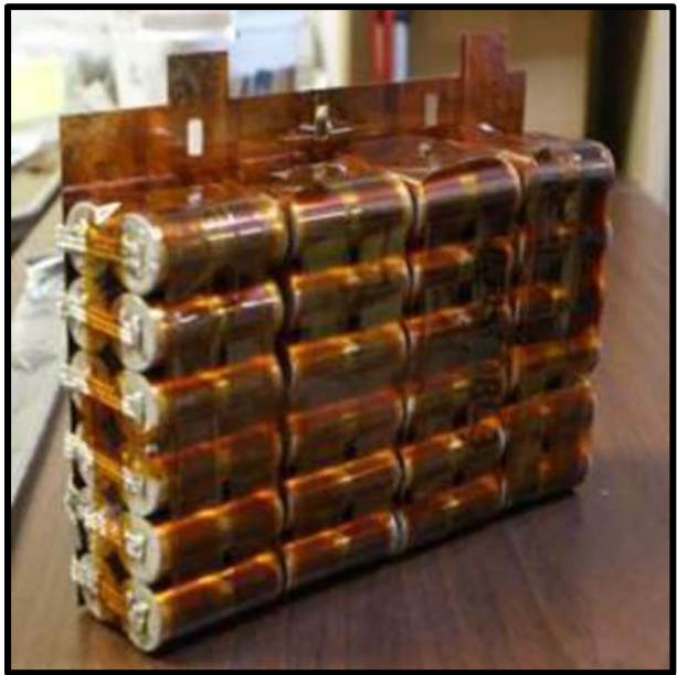
800 \mu F Extruded PEI Film Bulk Capacitor
