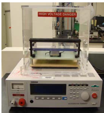
Figure 8. Dielectric resistance tester (Photo credit: Doug DeVoto, NREL)
