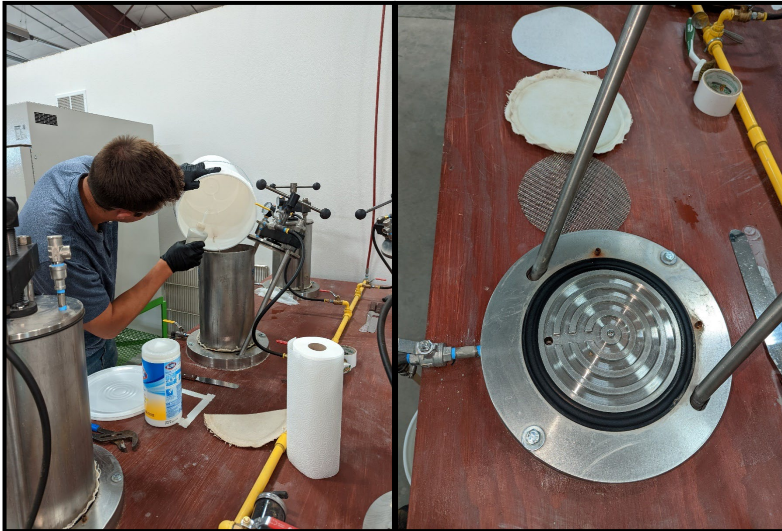
Figure G-1. Pressure Filter Apparatus at the Disa Process Laboratory Used for Removing Water from the Passing 270-Mesh Fraction after Wet Sieving with All Components Laid Out on the Table
