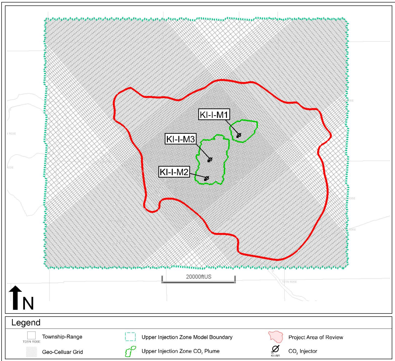
Figure 3.3a. Plan view of the Upper Injection Zone model boundary and geo-cellular grid used to define the CO 2 plume extent and associated project AoR.
