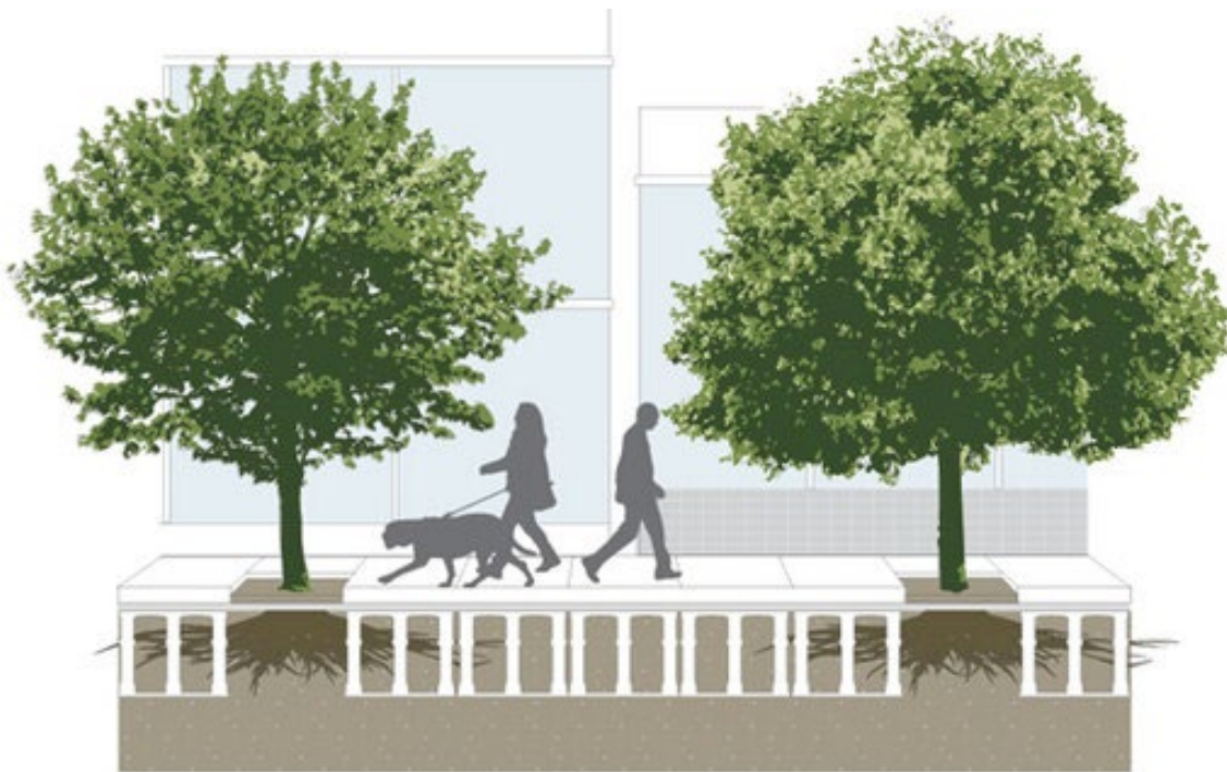
Figure 2. Example of suspended pavement system. Source: https://www.landscapeperformance.org/blog/2015/06/tracking-silva-cell-tree-performance
